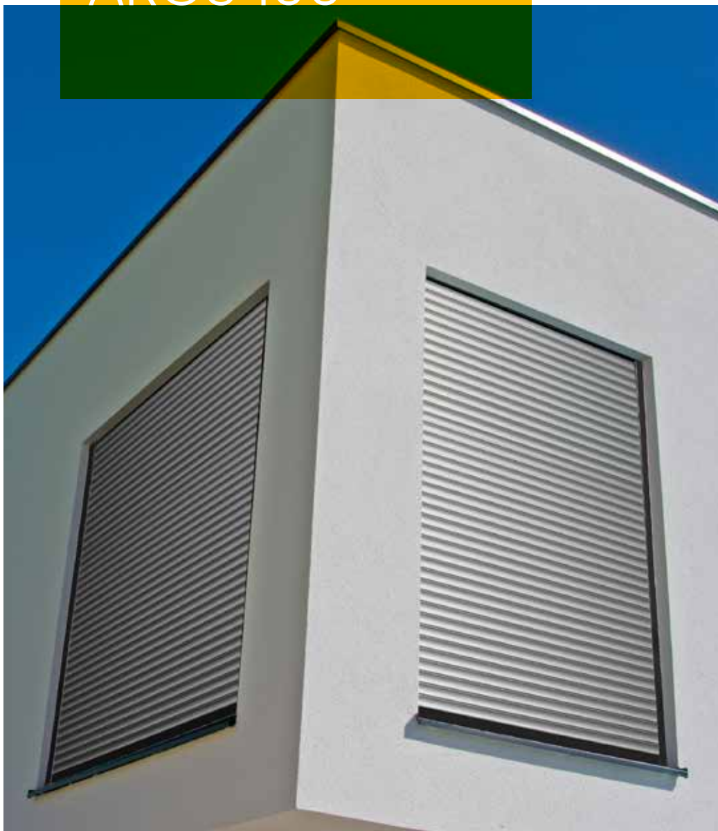
AROS 100 Roller shutter without headbox cover for installation in an existing recess. Max. width 3000 mm Max. height 3500 mm
